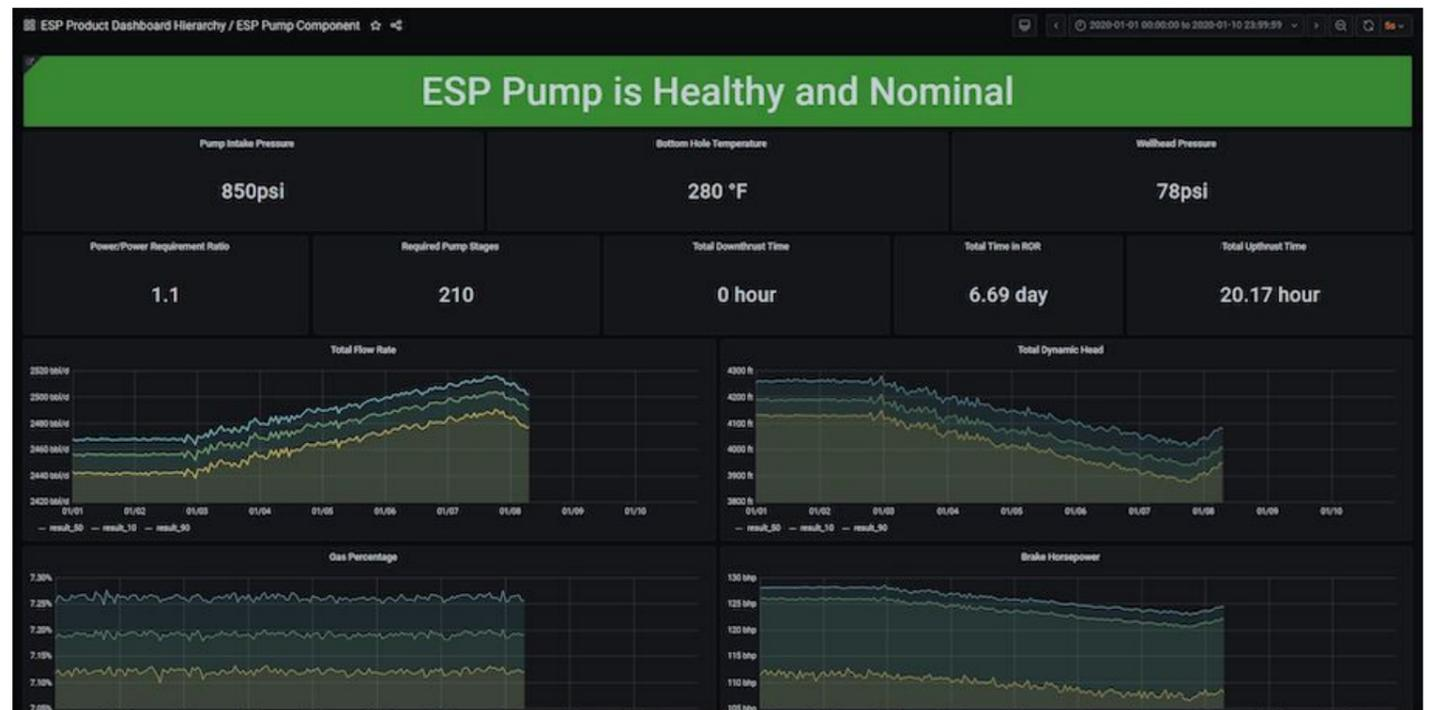
Lone Star's MaxUp analytics software maximizes uptime by mitigating issues before they happen on up to 60 different failure modes and predicts when a replacement is required so the proper personnel, equipment and tools are available at the right time. (Source: Lone Star Analysis)
