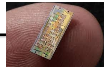
Xanadu's nanophotonic chip powered by laser pulses
